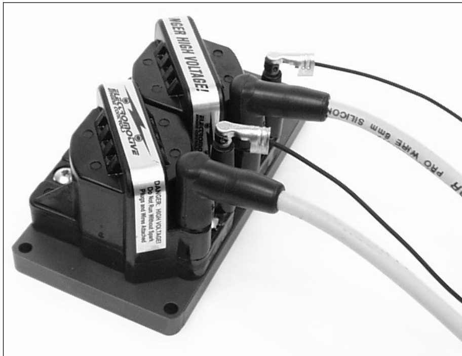
Fig C.2 1: Ground wire installation for coil-per-plug (non-waste spark) applications. Note that the 16awg wire attached to the unused coil terminals should ground to the engine block.
